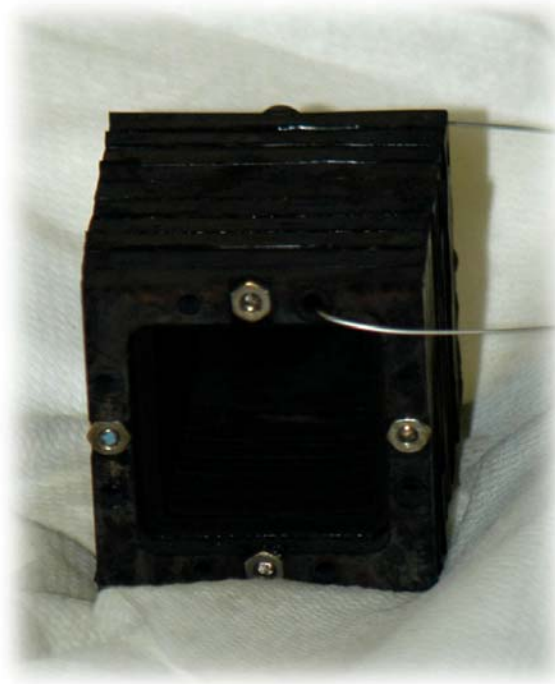
Figure 9. Inner baffle after application of Ebanol C.
